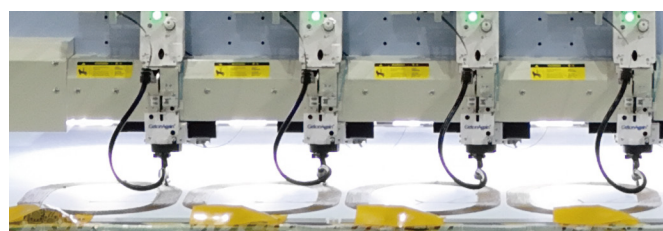
气动夹框：自动夹布，夹持牢固；具有夹持、拉伸功能，保证布料平整无褶皱 Pneumatic Clamping Frame: Automatically clamps the fabric securely and provides both clamping and tensioning functions to ensure the fabric remains flat and wrinkle-free.
